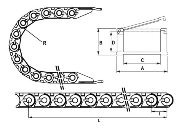
Full length = 1000mm Inside Height = 14.5Inside Width = 40Link Length(Pitch) = 20Outside Height = 20Outside Width = 49Radius = 028
